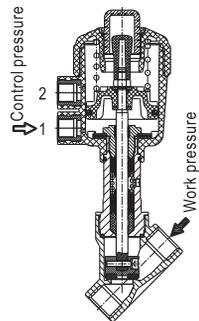
The working medium flows to the upper side of valve inlet
