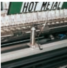
Winding diameter measuring at the laminating machine
